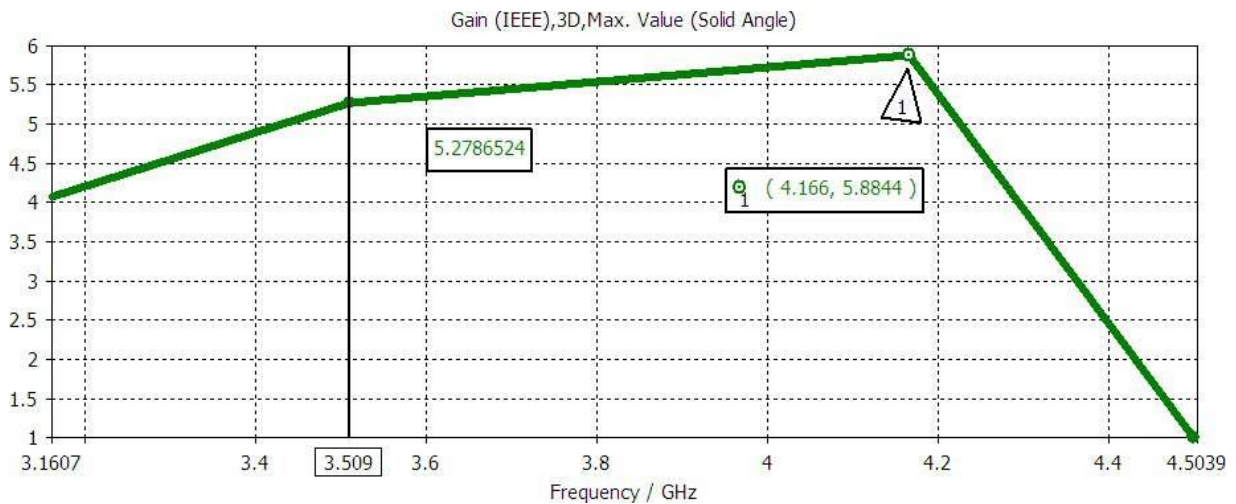
Fig. 12 Gain of the final proposed antenna at resonant frequencies 3.509 and 4.166 GHz respectively.
